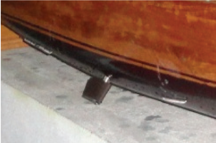
Figure 2. Installation of stabilizer to the model
