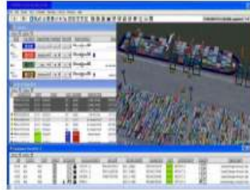
Simulation model (Virtual Terminal) connected to the TOS (Terminal Operating System)
