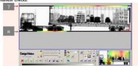
2D x-ray and Ray detection (Source: Smiths Heimann GmbH)
